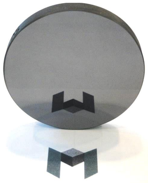
Figure 8. Example of directly polished RBSC 100 mm diameter disc (12 µm grain size)
