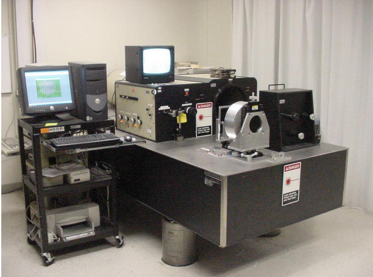
Figure 4. The overall system. The 1 inch output is dead center. The subsystem (rear view) is between the two Danger Laser placards. The 12 inch aperture collimator output and return mirror are on the right, unused in this application.
