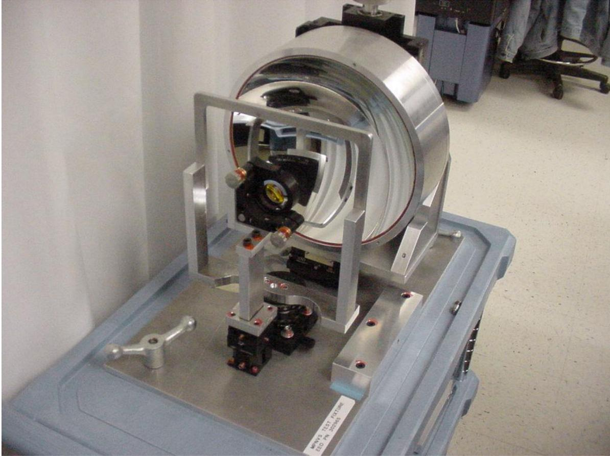
Figure 9. Interchangeability. The subassembly removed and placed on a cart for temporary storage. Removal and replacement are a snap and do not require realignment.
