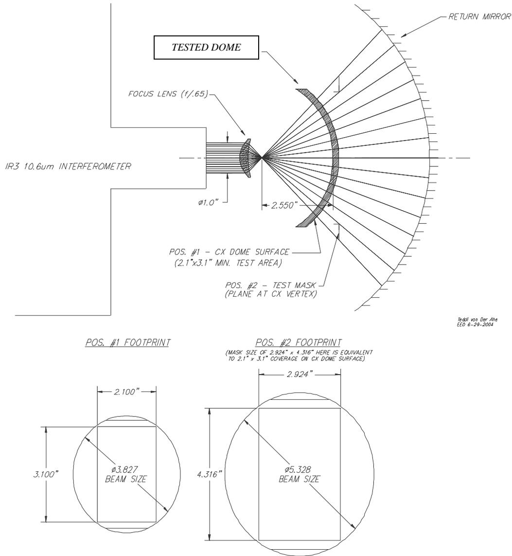
Figure 2. Optical element geometric layout, and test aperture definition.
