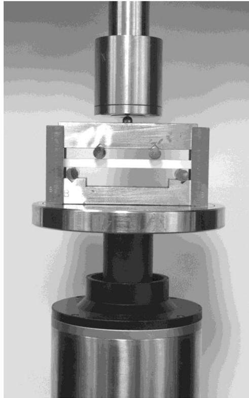
Figure 3: Four-Point Flexure Fixture loaded in the Instron Universal Tester
