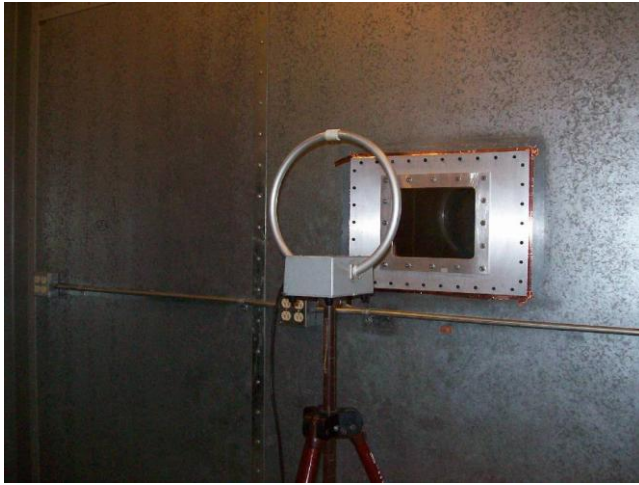
Figure 6: Loop antenna setup with the receive antenna shown.
