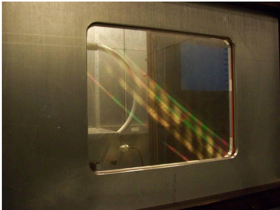
Figure 4: The window is put in place with the conductive gasket making contact with the buss bar and the fixture. A non-conducting gasket and retainer are placed on the opposite side to sandwich the window in place.
