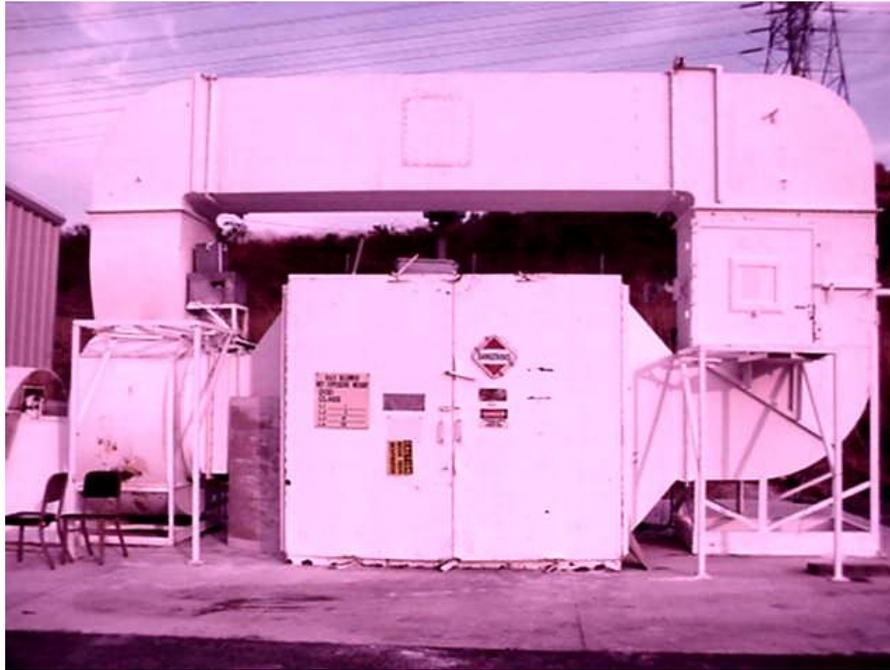
Figure 3: Example of a blowing sand test chamber
