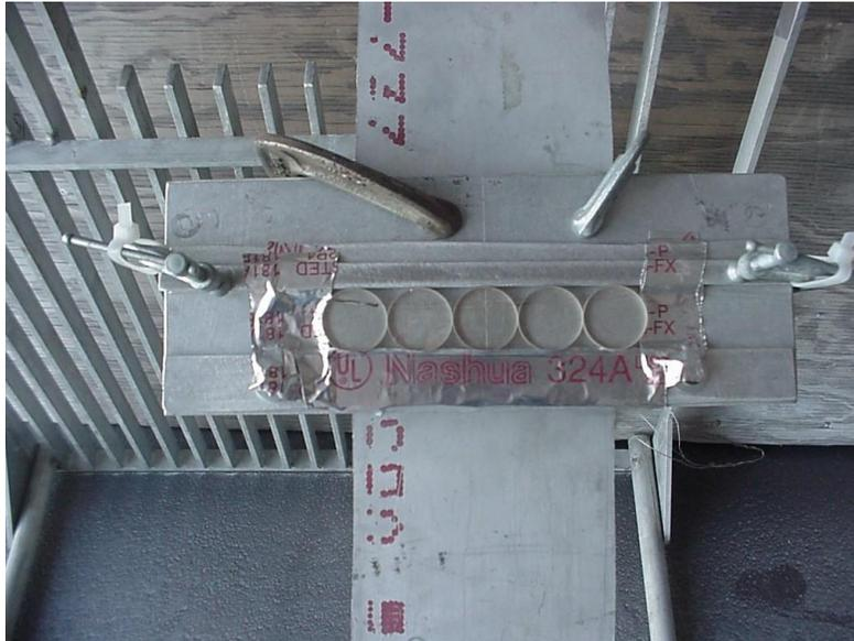
Figure 5: Example of a way to mount the test samples (samples shown are property of EEO)
