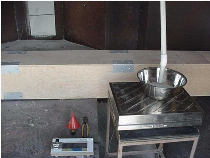
Figure 6: Example of a mass flow rate calibration set-up
